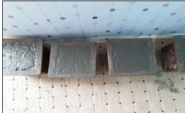
Figure 2. Casted concrete cubes
